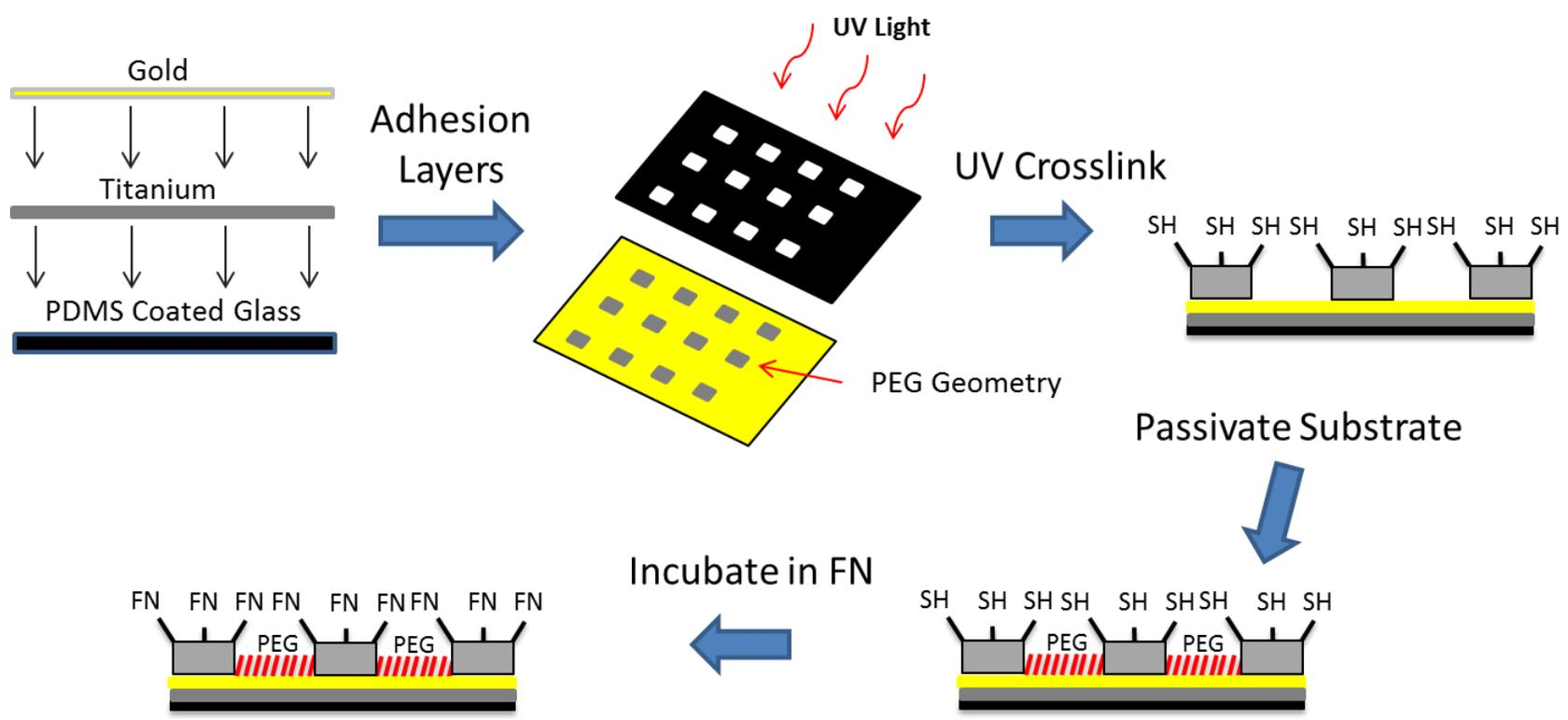
Figure 5.3: Schematic showing UV lithography process used to create hydrogel shapes of varying elasticity. Hydrogel shapes were functionalized with thiol to promote fibronectin binding exclusively to hydrogels.
