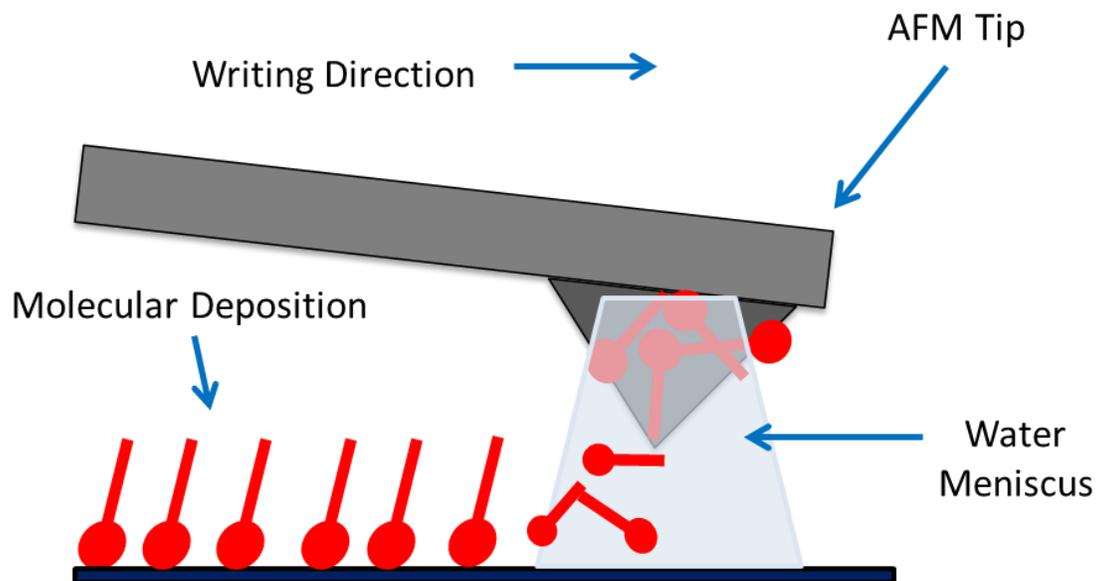
Figure 3.2: Schematic of DPN process. A single DPN tip coated with molecules deposits the “ink” via a water meniscus onto the surface in a nanopatterned array.
