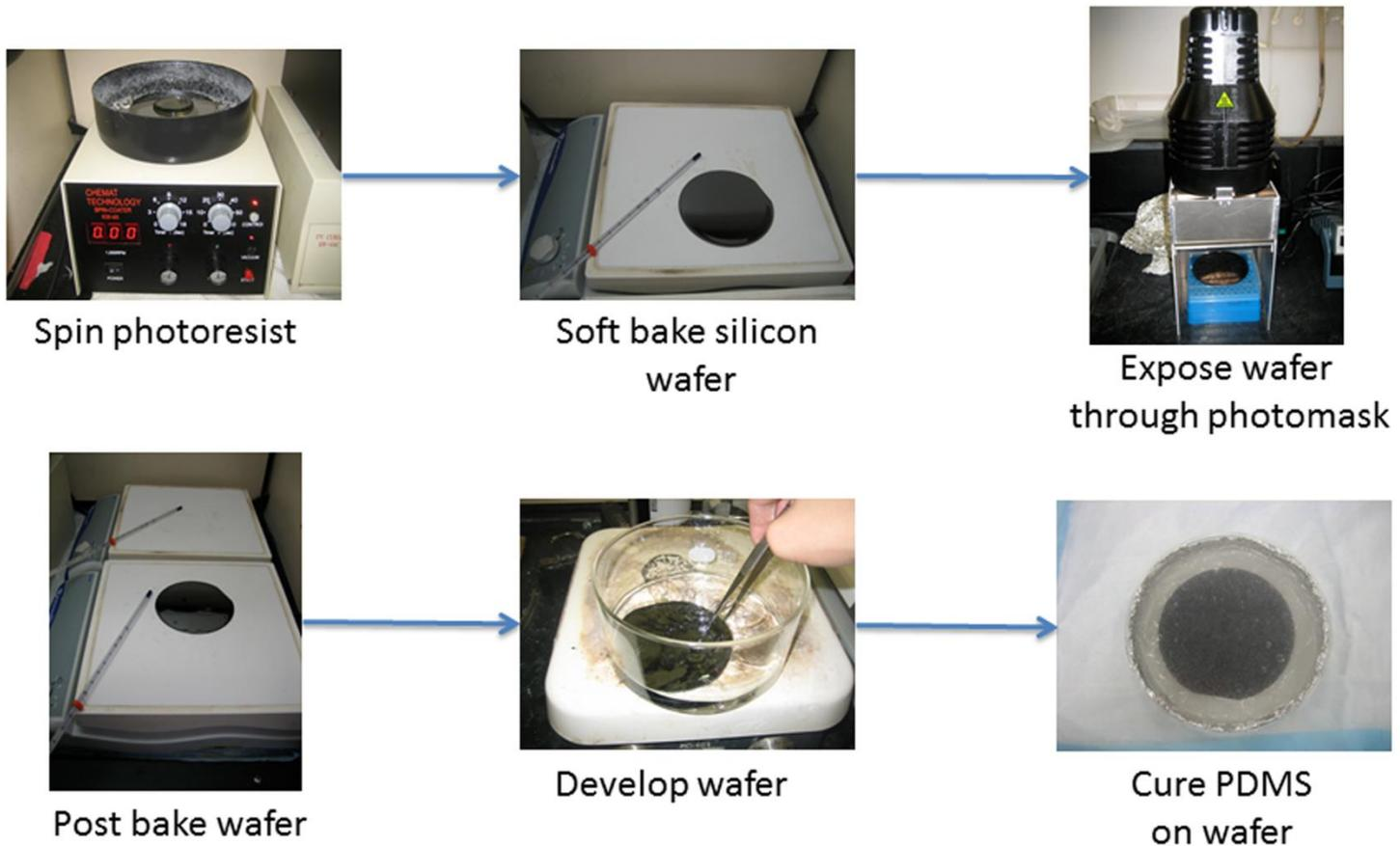
Figure 3.8: Schematic showing the procedure for development of microfluidic channels. First photoresist is spincoated onto silicon wafer at desired thickness and wafer is soft baked for recommended time. Wafer is then exposed to UV light through a photomask to pattern desired features into photoresist and post baked. Wafer is then developed to remove uncured photoresist and PDMS is coated onto developed wafer to make microfluidic channels.
