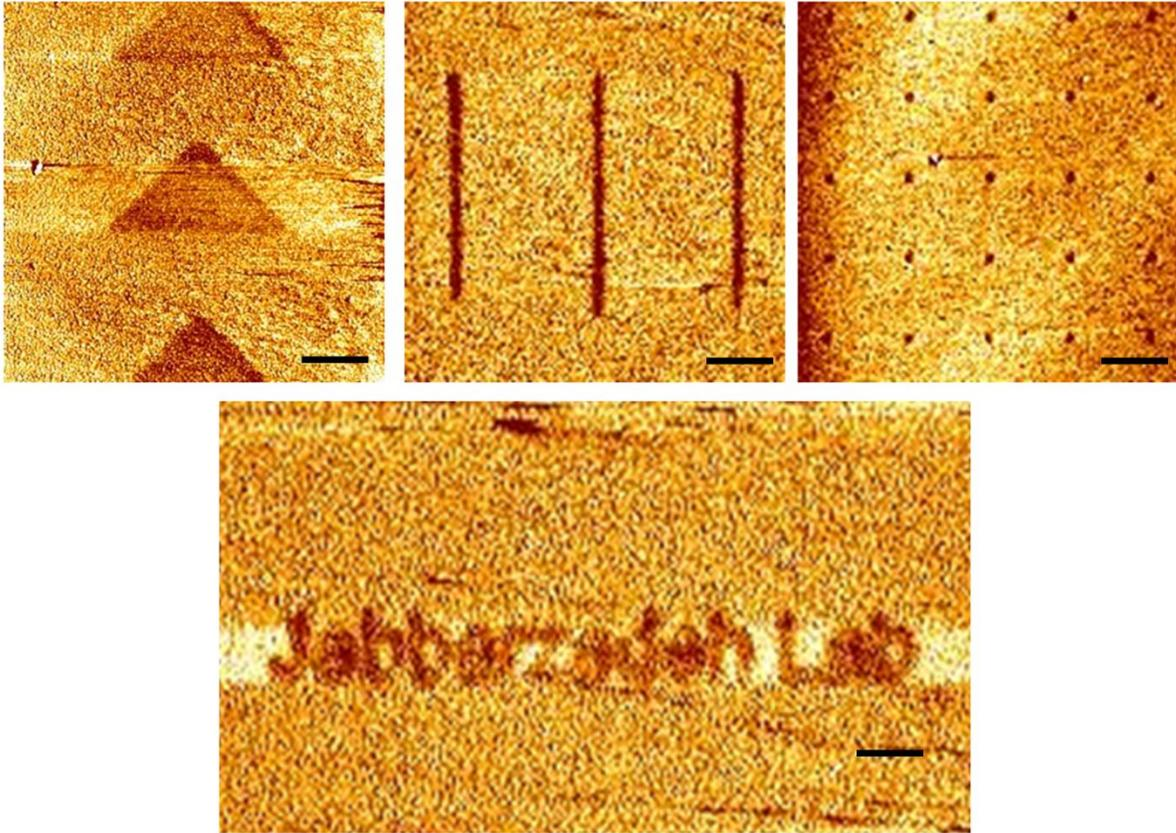
Figure 3.3: Dip Pen Nanolithography is a scanning probe lithography used to deposit substances onto a surface through an atomic force microscope tip. Shown here is alkane thiols printed onto a gold surface. (A)-(C) Triangles, lines, and circles respectively and (D) “Jabbarzadeh Lab” printed out in alkane thiols. Scale bars are 500 nm.
